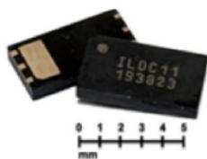
ILDC11-15E Ultraminiature Isolated DC-DC Converter
