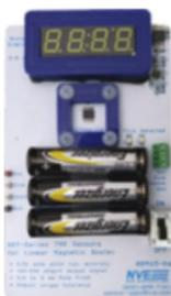
The [AG970-07E Evaluation Kit](#) helps test AET-Series sensors with magnetic linear scale tape. The kit includes:
